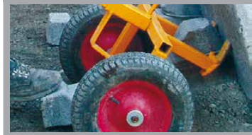
LOCK+LOAD CHARIOT DE MANUTENTION
